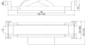
Electrohydraulic lift for geometry • platforms with grooves for turntables and expansion plates • mechanical height lock released pneumatically • adjustable position of one platform • perfectly secured hydraulic actuator • galvanised ropes initially stretched • rope wheels with large diameter • lift lock while slackening or breaking ropes • lift steering with safe voltage 24V • safe device compatible with norm EN1493:2010.
